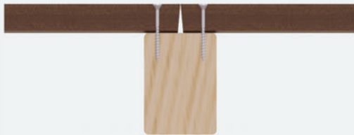
Slightly undercut for tight jointing
