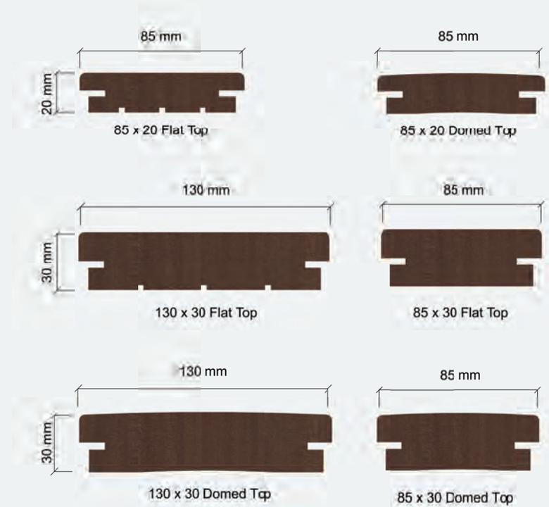
**Metroplank™** offers both flat and domed top option. Flat top is generally used in areas not exposed to the weather, however if exposed a 85×20 or 85×30mm are recommended. Domed top was designed for maximum durability, the domed surface provides maximum water run-off keeping the timber dry and stable.
