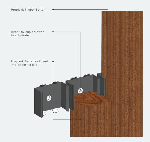
Direct fix clips are used where the Proplank mounting rail is not required. The clip allows battens to be fixed directly to the substrate
